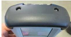
**B.** Place new cover onto the exposed enclosure. The new holder will slide right on. Layout GPS, Screws, and extended cover for next steps in the installation.
