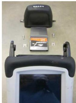
**C.** Here the user can see the two exposed ports. The two hold clips and Screws have been installed.
