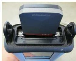
**E.** Place on extended cover and lock each side to securely fix to Recon housing.
